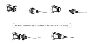
Insert plug into light and secure with screw-on cap
