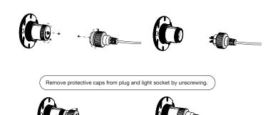
Insert plug into light and secure with screw-on cap
