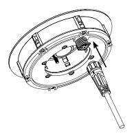
3. Connect PAL Bubbler Power Cable to PAL Bubbler LED Unit. Hand tighten nut.
