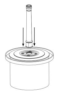
4. Install PAL Bubbler LED Unit into niche. Secure with 4 x #6-32TPI 3/4" stainless screws Optionally, push snorkel into Bubbler Unit.
