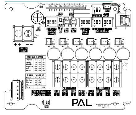
The 3D and 3DMX High Powered control boards feature additional dip switches for additional modes and functionality.
