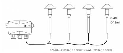
Daisy Chain Wiring (continuous run with taps to each fixture)
