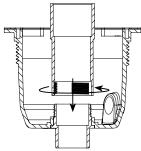
Before installing luminaire screw on internal pipe fitting.
