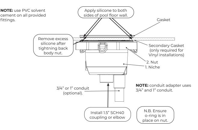
Except when the luminaire is installed in an area of the swimming pool that is not used for swimming and the lens is adequately guarded to keep any person from contacting it, the luminaire shall be installed in or on a wall of the pool, with the top of the lens opening not less than 457 mm (18 inches) below the normal water level of the pool. For supply connection, use only an isolating low voltage power supply with ungrounded output, evaluated for swimming pool use.
