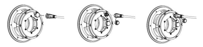
Insert plug into light and secure with screw-on cap.
