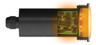
Traditional pool lights contain an integrated driver, which generates significant heat and requires water cooling. **High heat leads to premature failure.**
